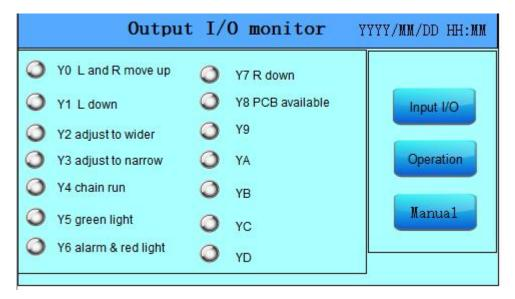
This page can view the REAL-TIME STATUS of PLC input and output
